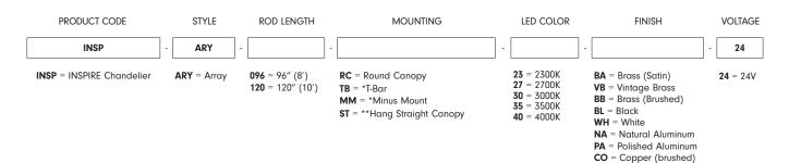
\*Factory standard 72" cable with **RC, TB, MM**\*\*Factory standard 24" Hang-Straight rod with **ST**
